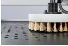
**10-SERIE-1300-MG:** The Manual Grinder is the cost-effective alternative to conventional grinding and deburring. Its head, consisting of a grinding wheel and a flap brush is tiltable about 180°. This makes it possible to the exchange between the aggregates easily.
